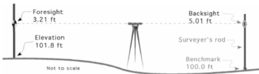
Fig. 15.3 Foresight rod reading
